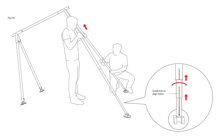
Note: Remove the bottom pin or pin nearest to the foot to expand the legs. Then replace pin when in desired position. Do not extend completely or legs will come apart or get jammed. A second pin will be required to extend the leg - if you over-extend the legs you will see a white stop cap - do not ever exceed this point.
