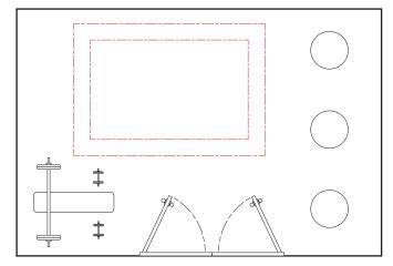
When the A-FRAME is at its lowest height, it will require a floor area of 4.4sqm (47 sq-ft) and when fully extended will require an area of 8.9sqm (95 sq-ft).
