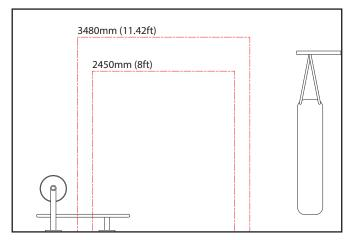
The A-FRAME could be extended from its lowest height of 2450mm (96.45 Inches) to a height of 3480mm (137.00 Inches) when fully expanded.
