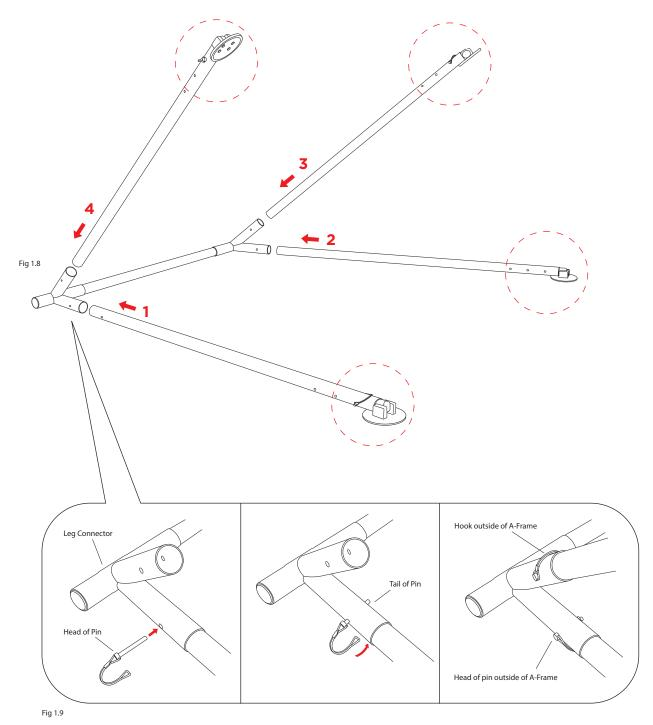
Note: Head of the pin on the outside of the legs and tail being on the inside.
