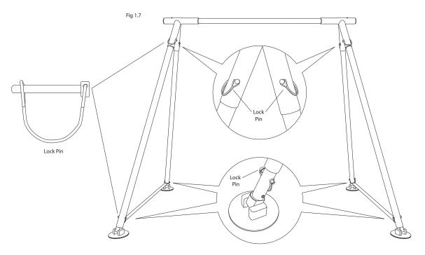
Note: Some pins come pre-installed on the A-Frame
