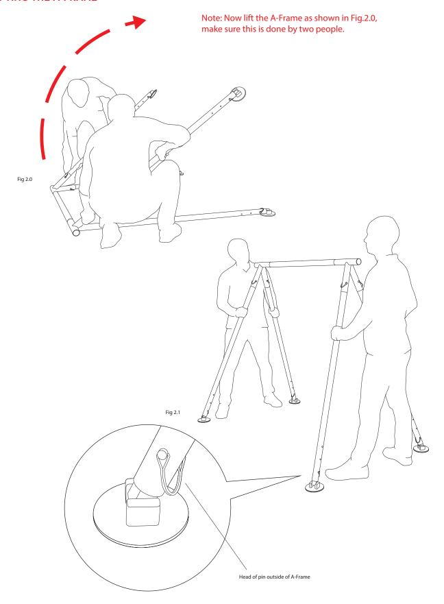
As the A-FRAME will be assembled on the floor and then lifted into position, it is important to allow enough space to do so. When lifted into position, make sure the feet are flat, by gently shaking the 2 legs each person is holding and slowly pulling outwards.
